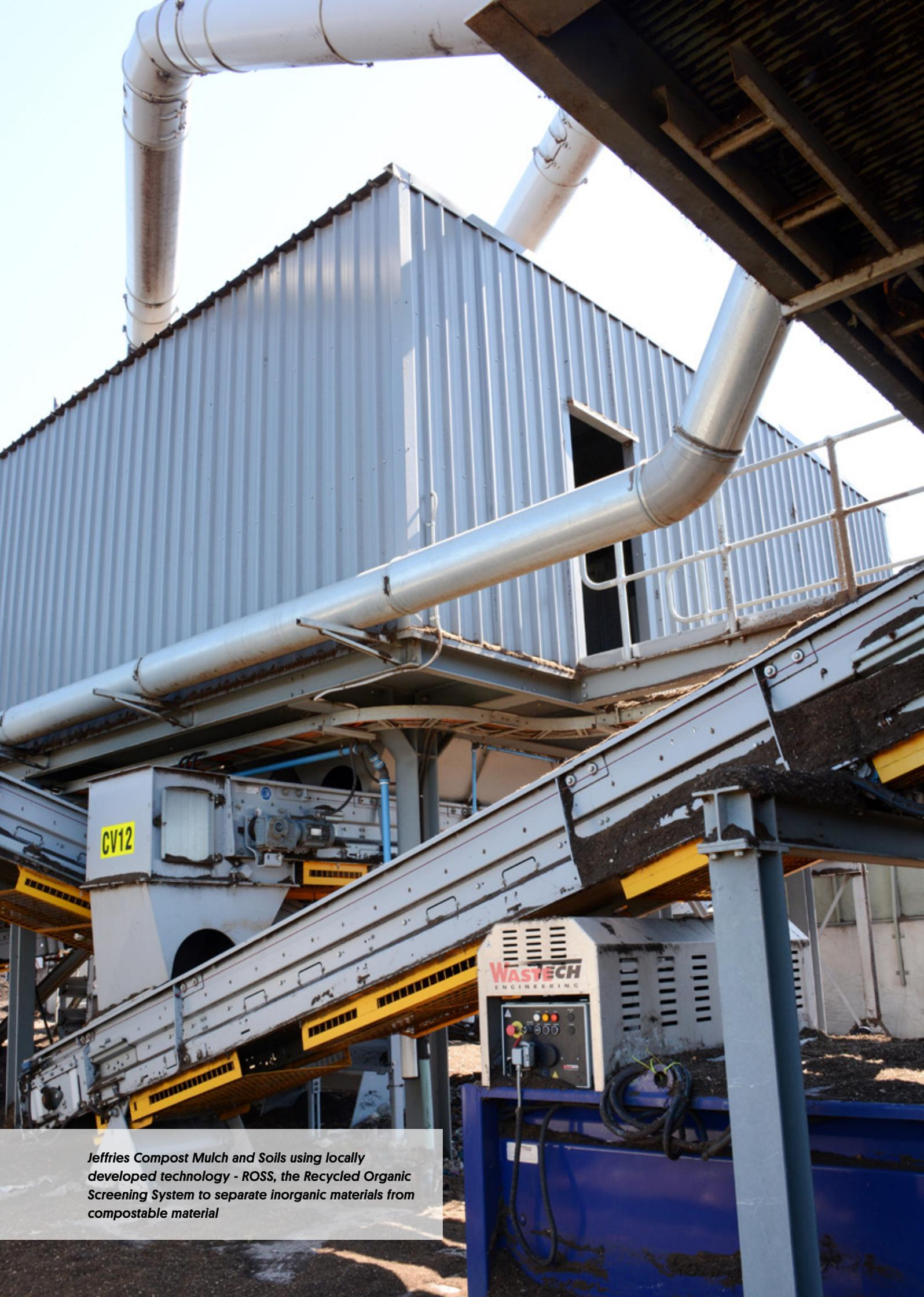
*Jeffries Compost Mulch and Soils using locally developed technology - ROSS, the Recycled Organic Screening System to separate inorganic materials from compostable material*
