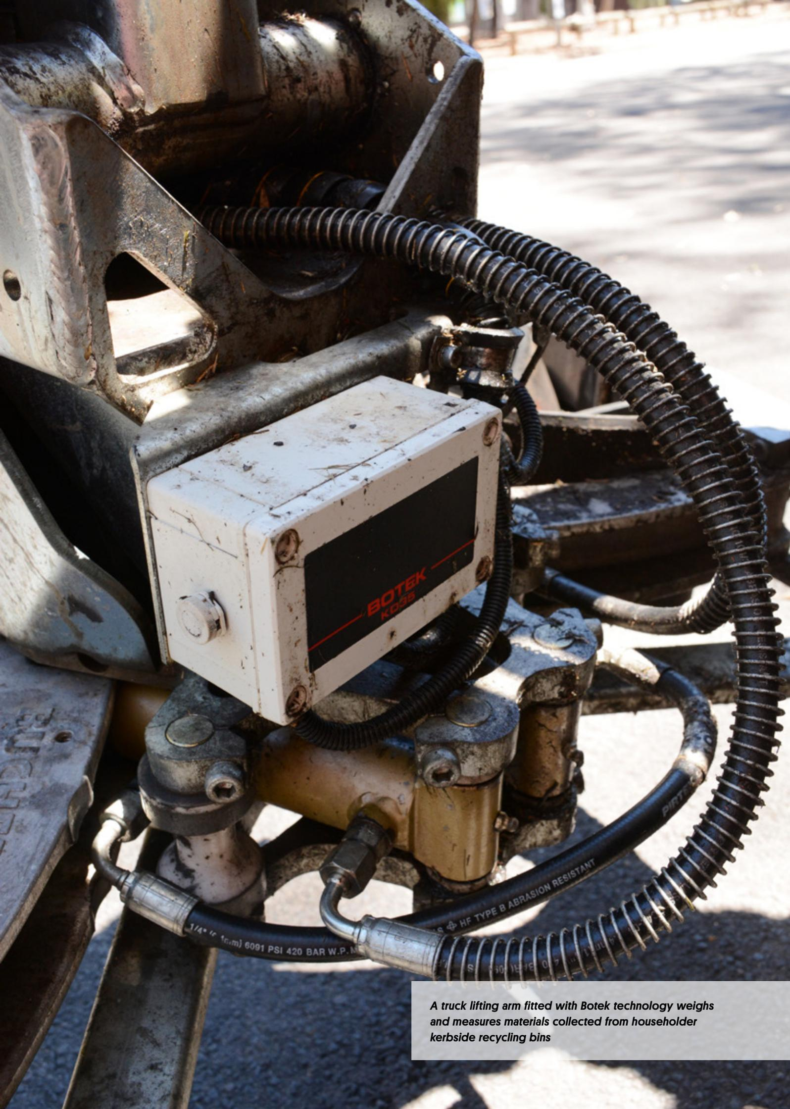
*A truck lifting arm fitted with Botek technology weighs and measures materials collected from householder kerbside recycling bins*
