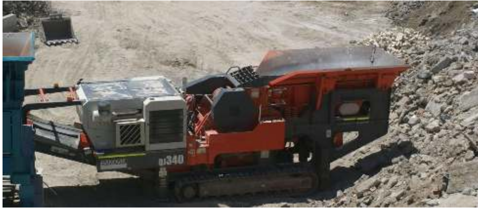
Figure C8.2: Mobile crusher (photo by Mike Haywood)
